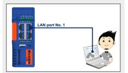
**2.2** Connect an Ethernet cable from your computer to the eWON's LAN port No. 1.
