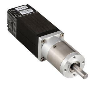
In addition to enhanced communication connectors, TSM11 StepSERVO Integrated Motors can be further equipped with planetary gearheads for applications demanding greater torque. The PH Planetary Gearheads offer ratios from 4:1 to 22:1, with additional ratios available upon request. These planetary gearboxes feature an all-steel gear train for long life and an attractive list price.
