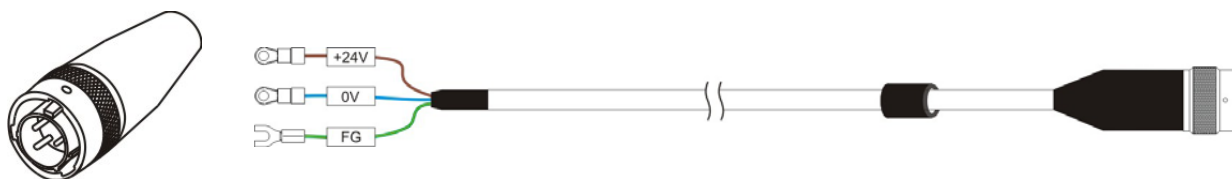
Figure 15: Male plug connector cod. UT0610-4PH (front view) and wiring.
