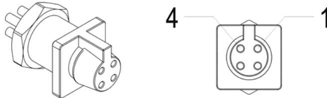
Figure 9: Female panel socket cod. 09-9766-30-04 (front view).
